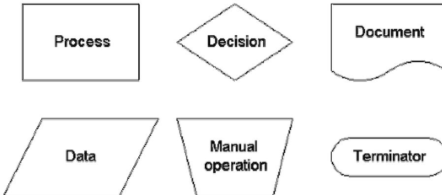
The next level of detail is to look at each process within the overall picture. The ANSI standard symbols used most often for this purpose include the following:
